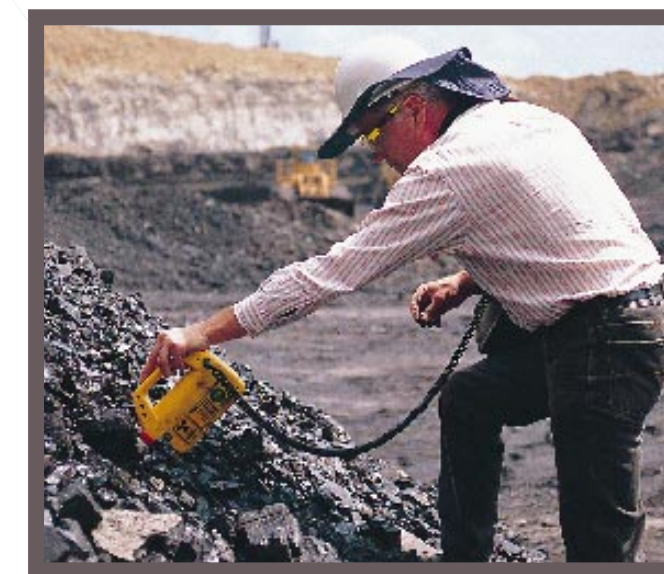
Mihai Borsaru examines coal ash content using the coal face ash analyser
