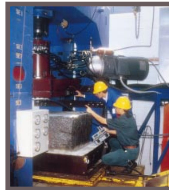
Oscillating Disc Cutter test rig (Image courtesy of CMTE)
