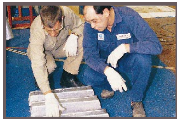
Simon Cashion and Nigel Ricketts discussing the surface finish of ingots cast under different protective gases (image courtesy of CASTMM)
